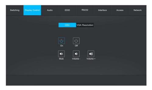
On the other hand, the VGA resolution page will allow you to select the VGA output resolution. You may select among 1024x768@60Hz, 1280x720@50Hz, 1280x720@60Hz, 1360x768@60Hz, 1600x1200@60Hz, 1920x1080@50Hz, 1920x1080@60Hz (Default) or 1920x1200@60Hz.
