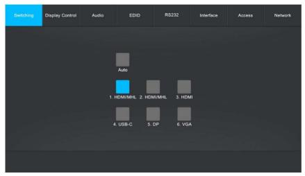
Clicking on the Auto button will enable the automatic switching mode. While the 1-6 buttons allows you to switch among the current connected sources.
