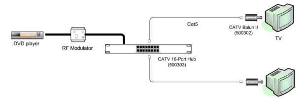
Figure 3: Typical Configuration, RF Modulation
