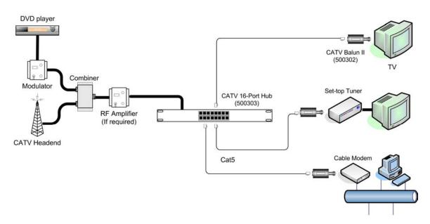
Figure 4: Typical Configuration, CATV & RF Modulation
