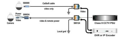
13. The 500124 is equipped with resettable fuses to protect the circuitry. In the event of a power surge, the fuse(s) will trip and the green LED will dim. In order for the fuse(s) to reset, the power to the 500124 must be turned OFF for 2-3 minutes. The fuse(s) will then reset and the power can be turned on again.
