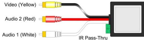
3. Plug the second balun into the composite video/stereo audio input of the video screen or receiver at the remote end.
