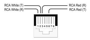
**Note**: The Stereo PC-Audio Balun is phase polarity sensitive. Therefore, in order to achieve full stereo audio quality, please ensure that the wiring is straight-through and according to EIA568 (A or B) standard.
